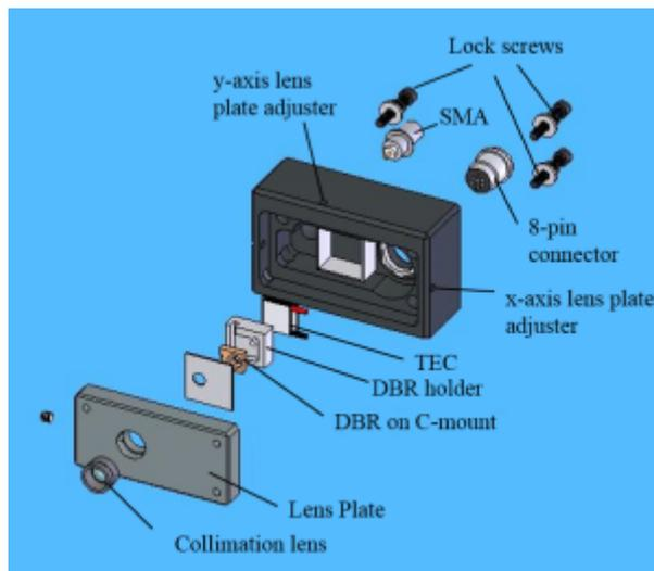
Fig. 2: Exploded view of the DBR subassembly
