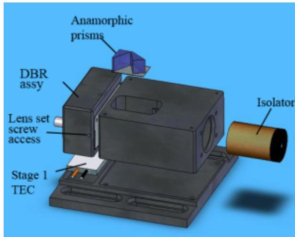
Fig. 1: The DBR Laser Module
