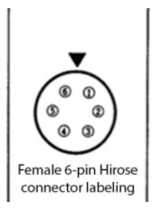
Fig. 1: Pin numbering on female Hirose 6-pin connector
