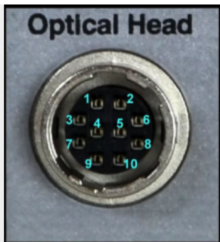
Figure 3: Pin-Out for the LC-105 connection to the optical head.
