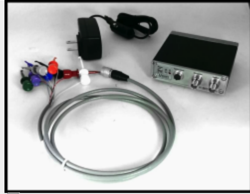
Figure 2: The LS-105, power supply, and connection cable. The figure above shows a cable for connecting to a chip-level SEEOR. For a fiber packaged device, the cable will have connectors on both ends.
