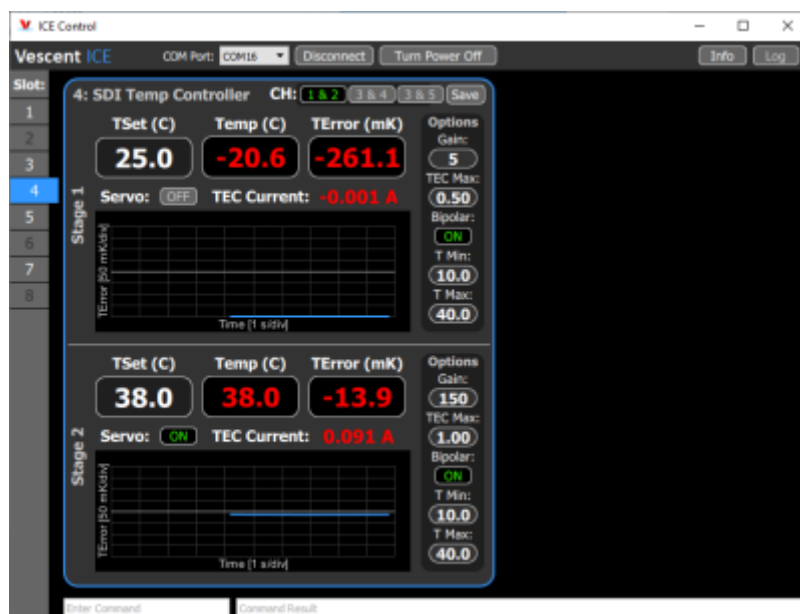
Fig. 10: A GUI representation of the Temperature Control Board with a plot of TERROR showing Ch 2 temperature stabilized and Ch 1 off.
