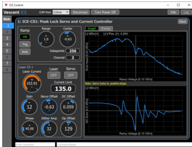
Fig. 12: A GUI representation of the Peak Lock Board.
