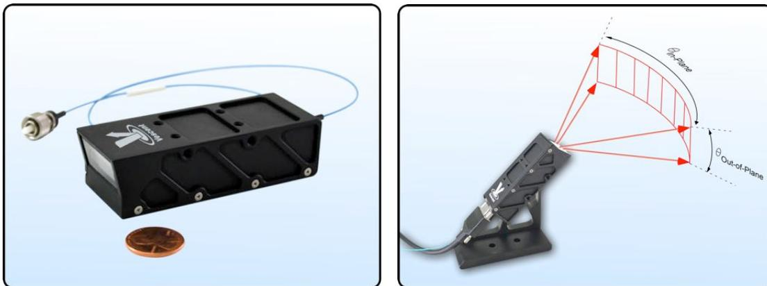
Figure 1: Pictures of simple, wide field of view EO scanners. LEFT) The optical head. A short-wave infrared beam enters the device through the single mode polarization maintaining fiber and an EO scannable beam exits through the window. RIGHT) The photonics package mounted and a cartoon depiction of the EO scannable field of view.
