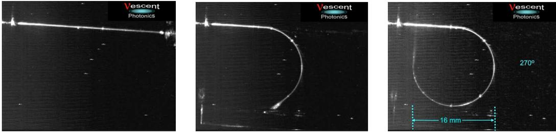
Figure 3: Example data from an electrode pattern that provided steering of 1550 nm light by 270° in a package that is smaller than a dime.
