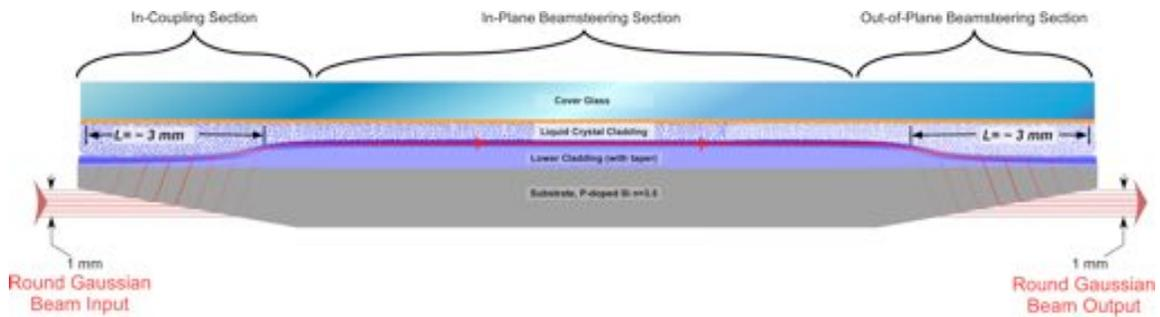
Figure 2 TOP LEFT) A 2-D electro-optic laser scanner. Voltage applied to the zig-zag patterned electrode (top left) provides in-plane scanning and voltage applied to the rectangular electrode provides out-of-plane scanning. TOP RIGHT) A picture of an EO scanner chip next to a quarter for scale. BOTTOM) A side view of a liquid crystal waveguide scanner. Integrated tapered-couplers provide both convenient coupling of round Gaussian beams and out-of-plane scanning control.
