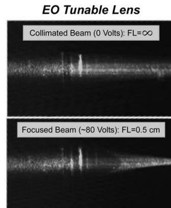
Figure 4: Operation of a voltage tunable lens.
