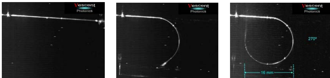
Figure 4: Example data from an electrode pattern that provided steering of 1550 nm light by 270 degrees in a package that is smaller than a dime.
