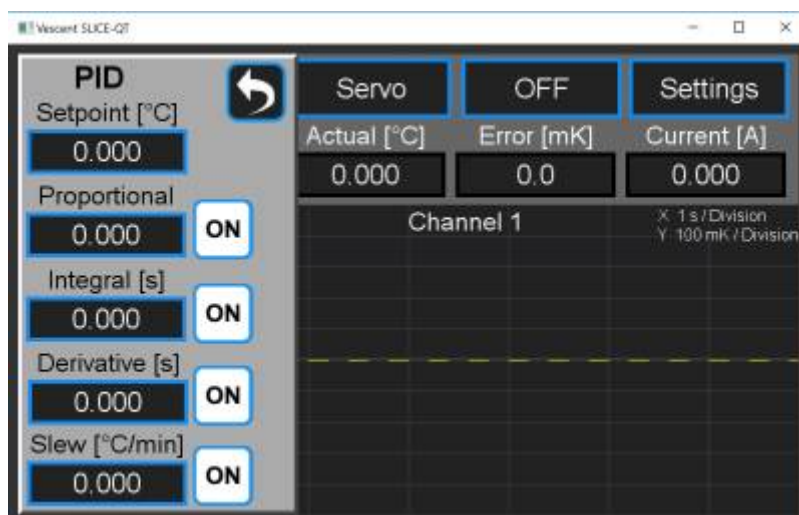
Fig. 23: Screen for adjusting PID parameters for individual channel
