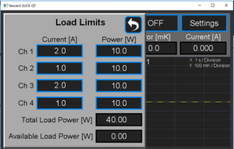
Fig. 25: Screen for adjustment of control power capacity
