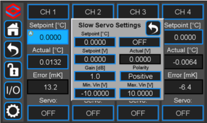
Fig. 31: Slow Servo menu showing adjustable parameters
