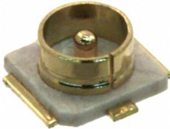
Fig. 7: Surface mount UMCC connector. Molex PN: 0734120110
