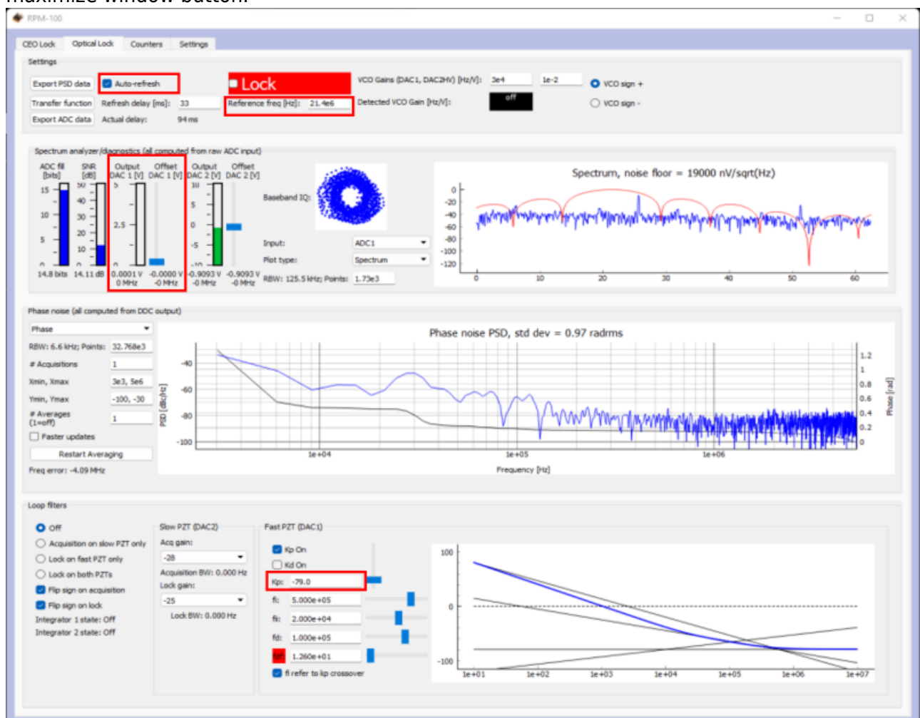
Fig. 11: Centering f(\text{opt}) on reference frequency (Baseband IQ optimization)
