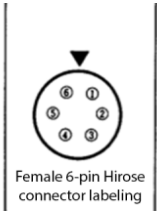
Fig. 3: Pin numbering on female Hirose 6-pin connector
