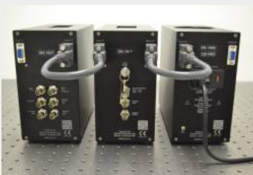
D2 Electronics with new-style power distribution cables (back view)
