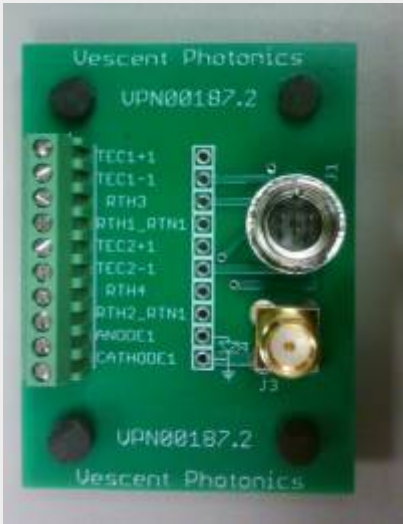
Fig. 1: D2-007 Breakout board.
